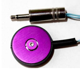
Figure 3. A C2 Tactor from Engineering Acoustics Inc.
