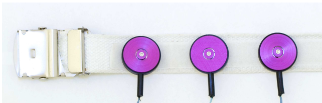
Figure 4. Belt lined with velcro used in experiment with 3 C2 Tactors attached.
